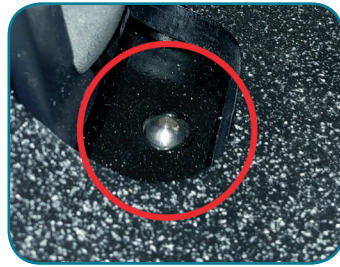
IMPROPERLY LOCKED INTO PLACE! DO NOT USE scooter
